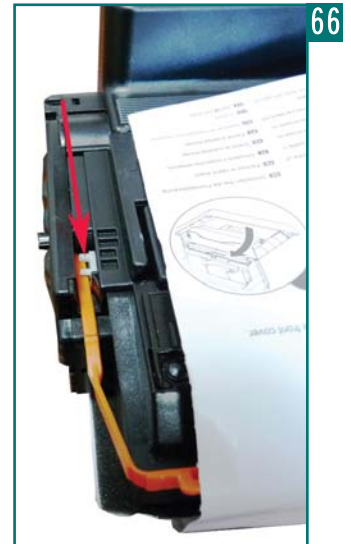
46 Install both sides of the PCR lock into the PCR holders as show. This lock keeps the PCR from touching the drum and will help prevent flat spots on the PCR during storage. See Figures 65, 66 & 67
