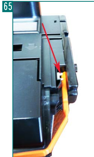
46 Install both sides of the PCR lock into the PCR holders as show. This lock keeps the PCR from touching the drum and will help prevent flat spots on the PCR during storage. See Figures 65, 66 & 67
